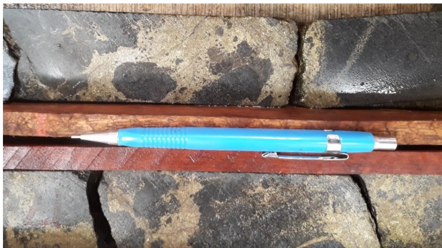
Figure 7-34: Typical brecciated mineralization showing angular pyroxenite clasts within a chalcopyrite matrix (MCSA, 2019)
