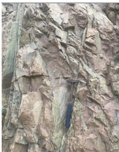
Figure 7-26: K-feldspar alteration of the ultramafic unit, south wall of the Cercado Velho open pit (Jacutinga, 2020)
