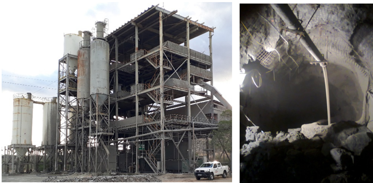
Figure 20-3: Paste fill plant on surface and underground tailings disposal as cemented paste (MCSA, 2020)
