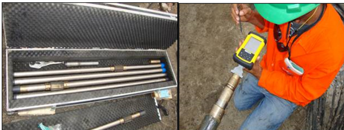
Figure 10-3: Maxibor equipment preparing for drill hole deviation readings (MCSA, 2018)
