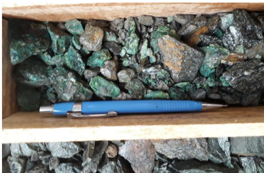
Figure 7-36: Malachite, typical copper mineralization in weathered zone (MCSA 2019)
