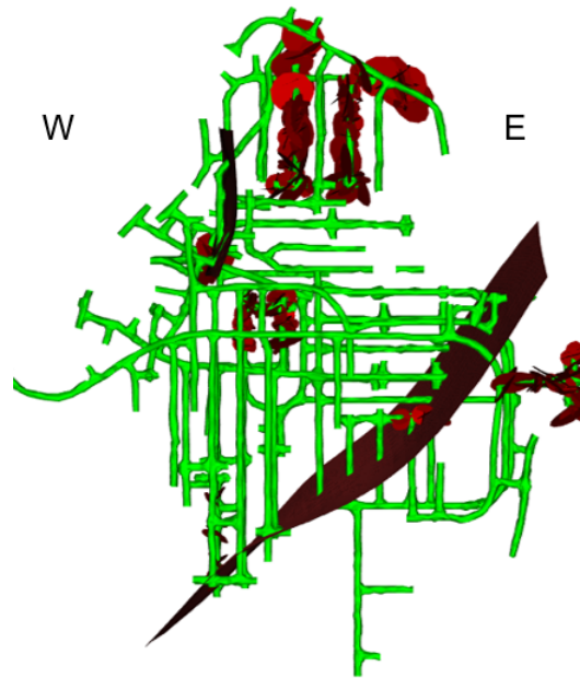
Figure 16-20: Structural mapping of Vermelhos Mine (red showing mapped discontinuities and green completed development) (MCSA, 2020)
