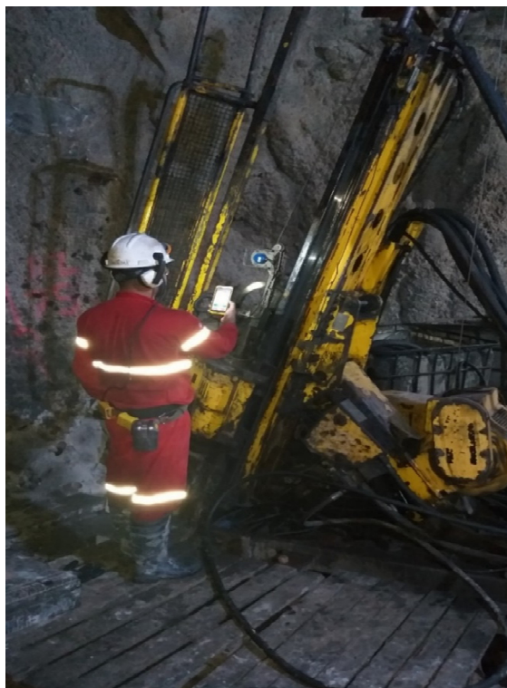
Figure 10-4: Giro Master equipment preparing for drill hole deviation readings (MCSA, 2019)
