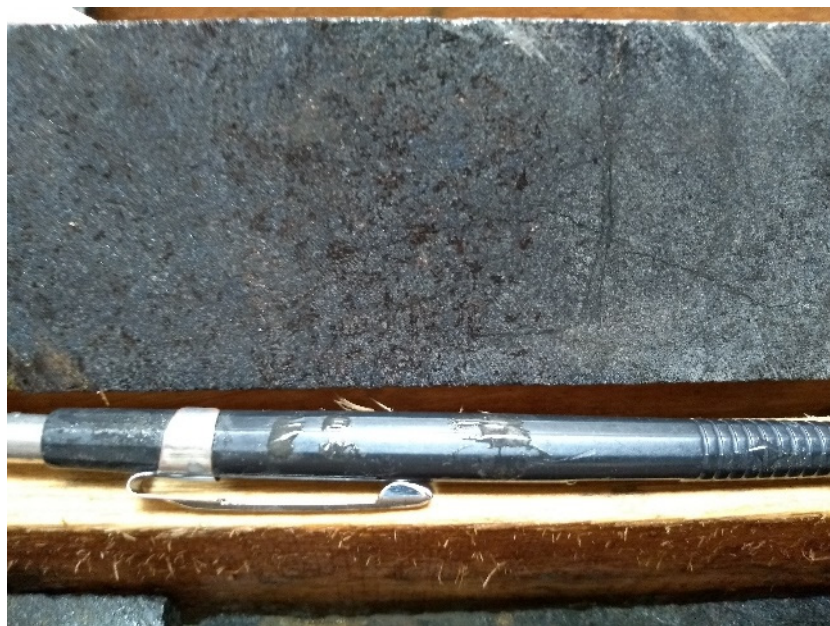
Figure 7-33: Typical disseminated chalcopyrite and bornite mineralization in pyroxenite grading to norite (right of the photo) (MCSA, 2019)
