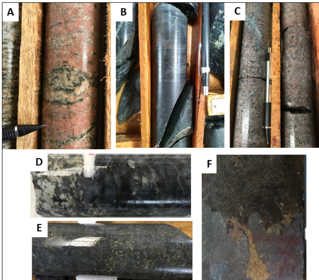
Figure 7-32: Alteration facies at Vermelhos mine. A) K-feldspar alteration overprinting gneissic fabric; B) Dark serpentinite alteration of ultramafic unit; C) Intense garnet alteration; D) Silica alteration on East side of the Vermelhos deposit overprinting the pegmatite unit; D) Silica alteration on East side of the Vermelhos deposit with disseminated chalcopyrite; and F) Phlogopite-rich alteration (darker) and pyroxenite (grey) with chalcopyrite veinlet (MCSA, 2019)
