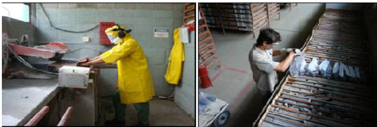
Figure 11-1: Core Sampling Procedures (MCSA, 2017)
