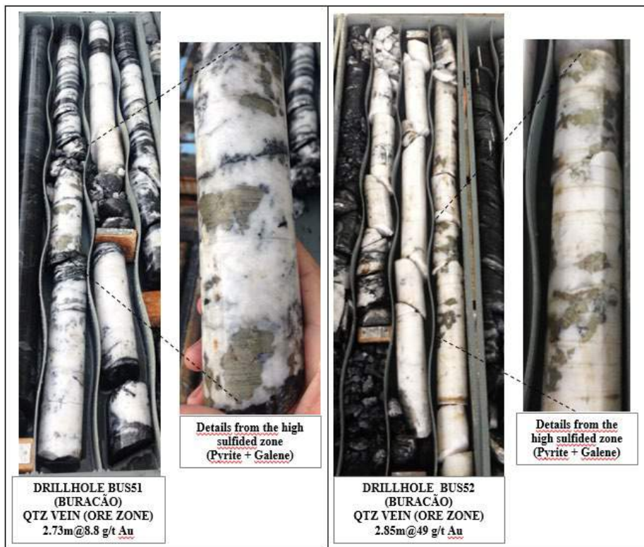
Figure 8. Quartz vein with high sulfadation (Pyrite and Galena) and high gold grade (NX Gold, 2018).
