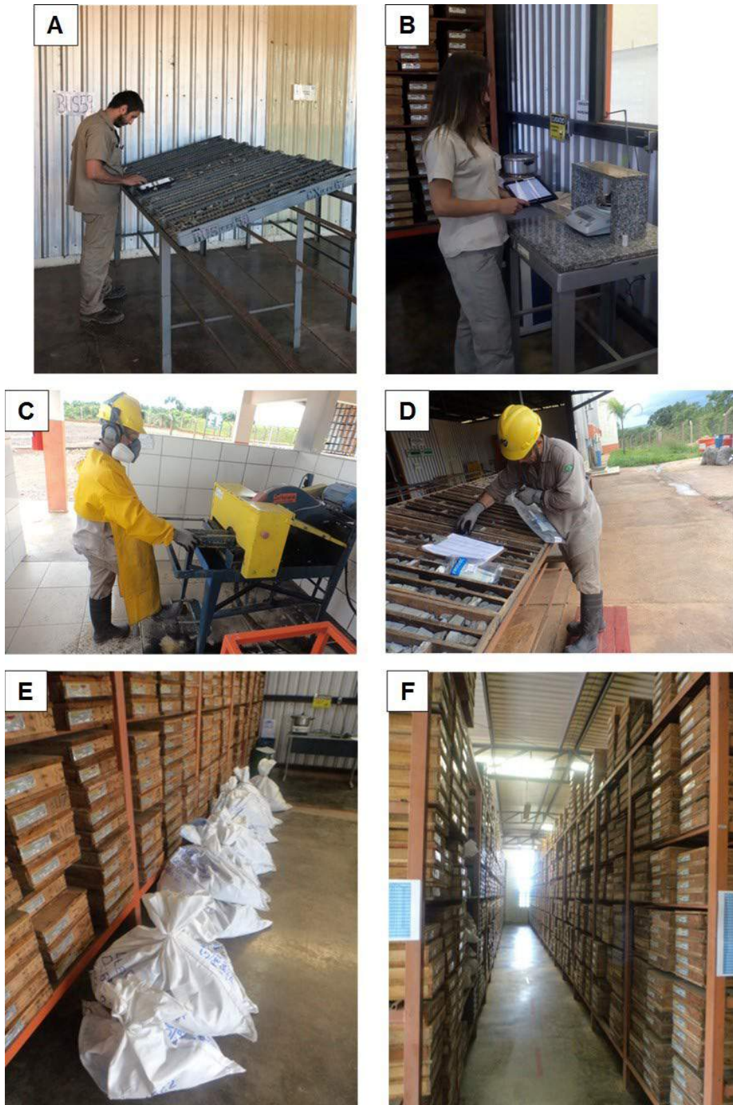
Figure 13. Pictures of the work site and standard operating procedure: (A) Geological description and geotechnical selection of the best intercepts for laboratory analysis; (B) Density Assay; (C) Cutting the rock cores; (D) Sampling; (E) batch ready to send to laboratory; (F) Hangar to file the core boxes (NX Gold, 2018).
