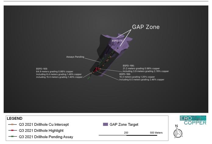
The center of the final pit design is located at UTM Easting 450722.00 and UTM Northing 9241657.00. The GAP Zone volume is shown to demonstrate a future area of exploration within the Boa Esperança final pit design. The shape is based on data compilation work which includes review of geological controls and structural analysis during the Company's technical programs. The interpretation and boundary limits do not imply continuity of mineralization or actual thickness of mineralization.
