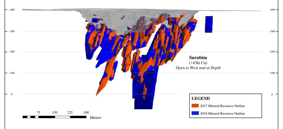
Mineral resource outline inclusive of mineral reserves. Amounts may not sum to total due to rounding. Incremental contained copper (000 tonnes) shown for Measured & Indicated mineral resource by area compared to 2017 Technical Report.
