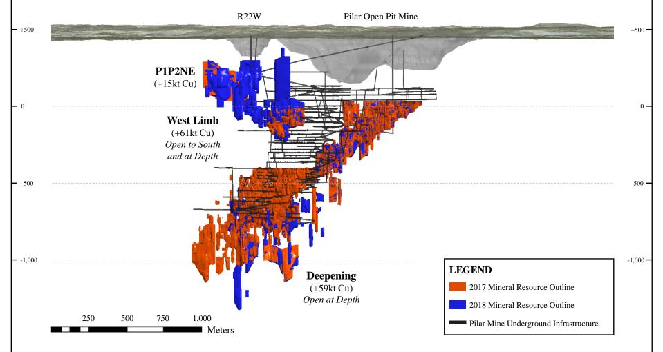
Mineral resource outline inclusive of mineral reserves. Amounts may not sum to total due to rounding. Incremental contained copper (000 tonnes) shown for Measured & Indicated mineral resource by area compared to 2017 Technical Report.
