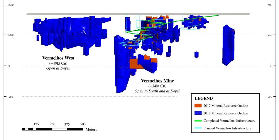
Mineral resource outline inclusive of mineral reserves. Amounts may not sum to total due to rounding. Incremental contained copper (000 tonnes) shown for Measured & Indicated mineral resource by area compared to 2017 Technical Report.
