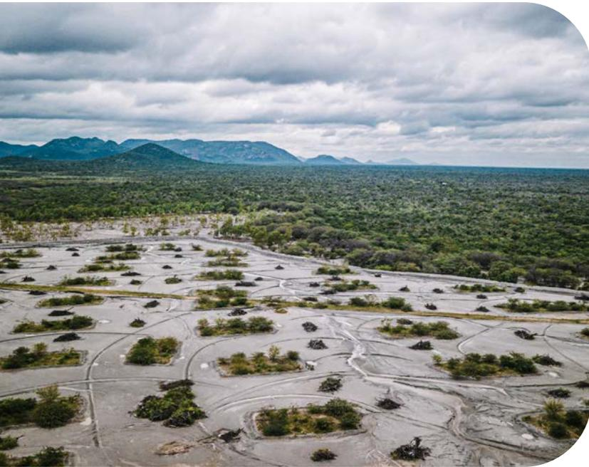
In addition to co-disposal methodology, Ero Copper has embraced the recent implementation of depositing naturally de-watered tailings – a geotechnically stable process that relies on the dry-climate and natural filtering of the material to dry tailings prior to deposition.
