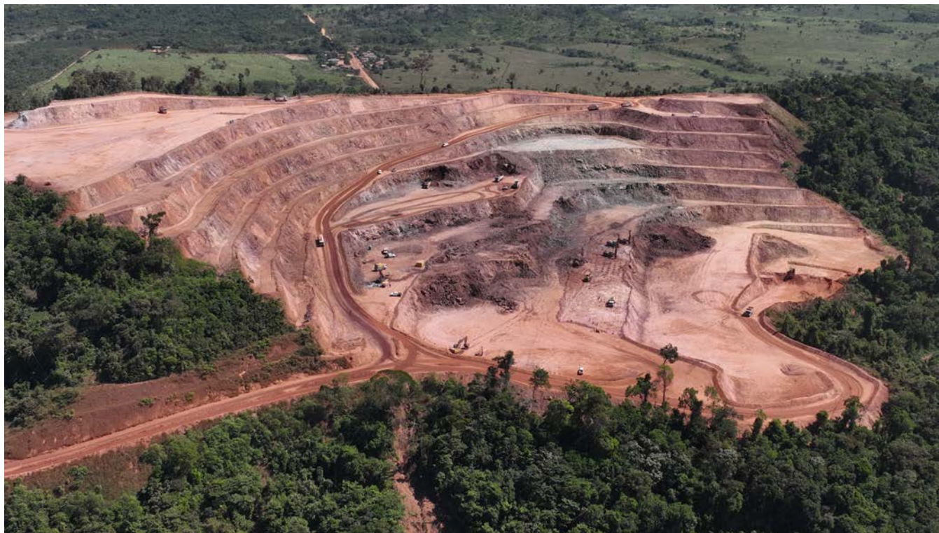
Figure 1: June 2024 aerial view of completed pre-strip and commencement of mining operations.
